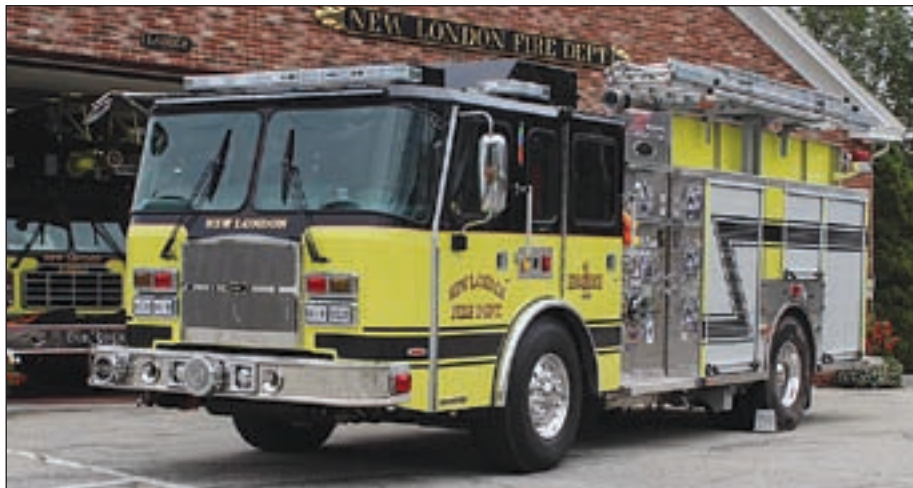
88 Engine 1 was recently delivered to the Town of New London. This multifunctional engine/tanker can pump 1500gpm and has the ability to transport water from a pond, cistern, etc. to the scene of a fire. The truck will go into service in a couple of weeks after the tools and equipment have been installed and the firefighters have been trained.
