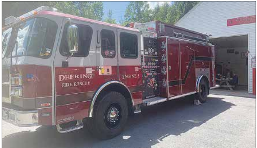
Deering Fire & Rescue took delivery of an E-ONE Typhoon with a 1500 gpm pump and 2,000 gallon water tank. For the next two weeks there will be driver and pump training. After that it will be put in service.
