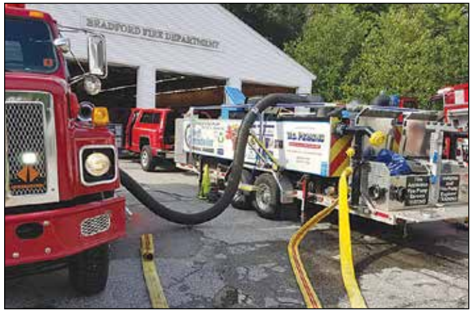
The Bradford Fire Department had two pumpers and one tanker run through their paces with yearly required pump testing.
